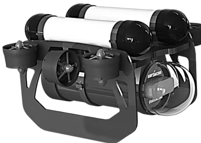
Fig. 1. Computer model of the developed underwater drone
